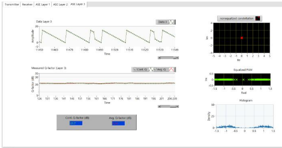
FIGURE 27. User Interface of Layer-3 Decoder of Three-layered ASE-DMT.
